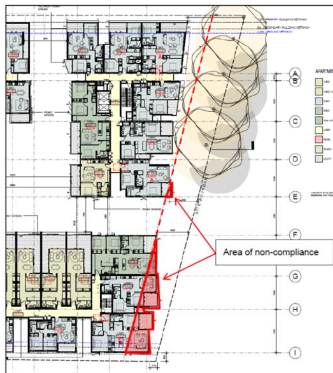
Figure 18: Building height standard non-compliance
